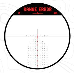
RANGE ERROR will display when the user ranges a target and a good reading was not received. This could be because the target is below the LRF's operating range (≤ 37 yards), the objective is dirty, or there is environmental interference (fog/rain/mirage). During a range error, a default aiming solution will display in the reticle for every 100 yard/meter increments up to 900 yards/meters (as is shown in the image).
