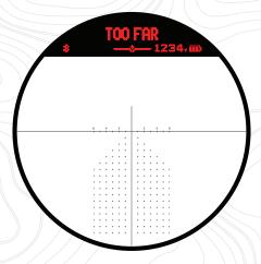
**TOO FAR** indicates that a firing solution cannot be displayed for your cartridge at any magnification.
