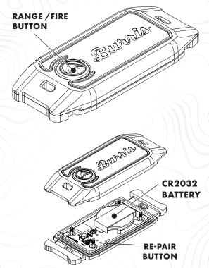
If the remote becomes un-paired, remove the screws from the back and locate the button under the cover. Press and hold for 5 seconds or until the HUD displays PAIRED.
