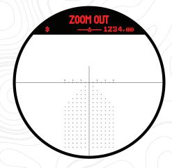
**ZOOM OUT** will display when there is not an aiming solution for the ranged distance at the current magnification. This occurs when the aiming solution is outside the field of view. Simply reduce the magnification until your holdover dot appears.
