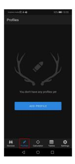
**3.** Create a profile for your riflescope, ammunition and zeroing distance. Make sure that "Ballistic parameters" switch is on. If your ammo is not on the list, you can enter its parameters manually. The more parameters you specify, the more accurate the recommended point of aiming will be.
