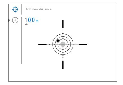
3. After adding the distance, it will switch to the **Zeroing parameters settings** menu —;— An auxiliary cross × will appear in the center of the display, and X and Y coordinates of the auxiliary cross will appear in the upper right corner.
