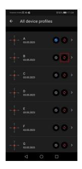
**8.** Set the status to "Active" for the ballistic profile. To do this, click on the button next to the desired profile, or select it in the profile selection menu in the riflescope.
