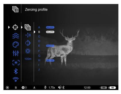
**9.** Make sure that the Ballistic Activation option is enabled in the riflescope's Ballistics menu.
