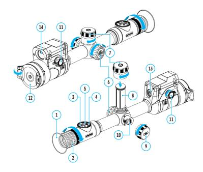
The riflescope is equipped with a built-in rangefinder (14), allowing you to measure distance to objects up to 800 m away.
