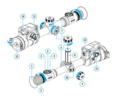
Magnification allows you to magnify via the device's digital zoom when zeroing, which reduces the MOA-per-click values of adjustments and improves zeroing accuracy.
